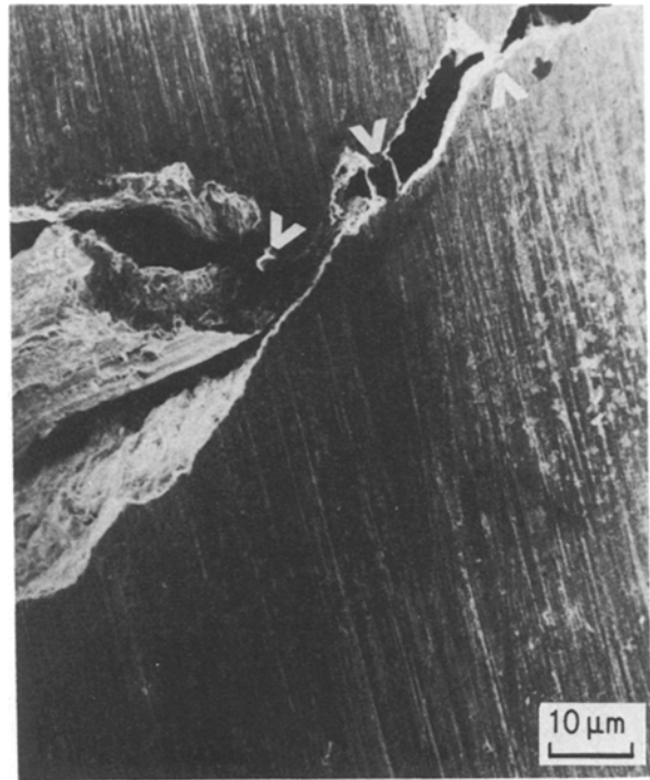
Figure 8 Cracks joining at inclusions. Arrows indicate inclusion locations.
